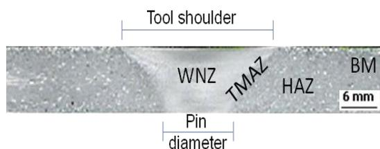
**Fig.1:** Macrostructure of friction stir welded joint
