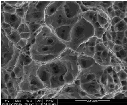
**Fig. 4:** Fracture morphology of FSW joints
