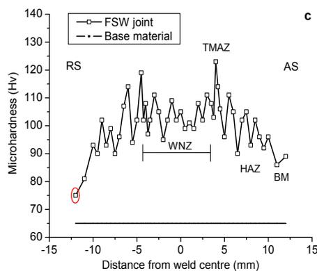
**Fig. 3:** Microhardness profile of FSW joints
