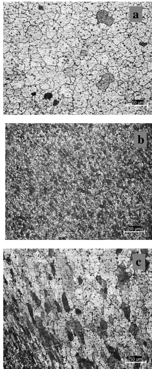
**Fig. 2** Microstructure of (a) base metal (b) WNZ and (c) HAZ of FSW joint
